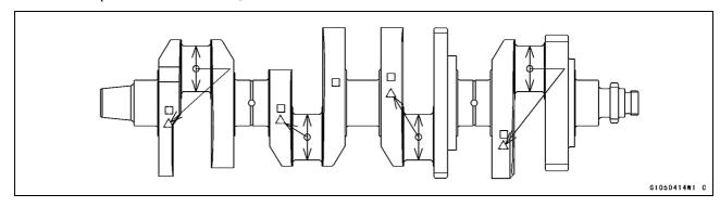
Measure the connecting rod big end bore diameter, and mark each connecting rod big end in accordance with the bore diameter.
