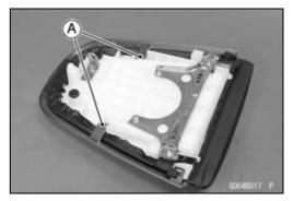
• Remove the front bracket portions [A] from the projection [B] of the seat.
