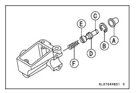
Rear Master Cylinder Disassembly
