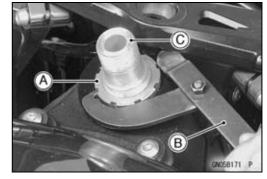
Drive out the bearing outer races [B] from the head pipe.
