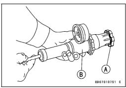
Watching the pressure gauge, pump the pressure tester to build up the pressure until the relief valve opens: the gauge hand flicks downward. Stop pumping and measure leak time at once. The relief valve must open within the specified range in the table below and the gauge hand must remain within the same range at least 6 seconds.
