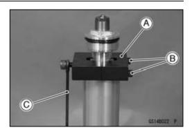
Olnstall the two collars [A] to the brake caliper mounting holes of the front fork bracket.
