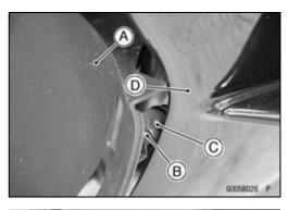
OPull out the lower fairings [A] to clear the its grommets [B] from the projections [C] of the upper inner fairings [D].
