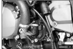
Remove the water pump cover [A] by inserting the screw driver to the pry point [B] on the water pump housing [C].
