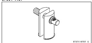
Valve Seat Cutter, 45° -  $\phi$ 35: 57001-1116
