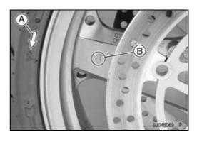
Before tightening the clamp bolts on the right fork leg, pump the forks up and down [A] 4 or 5 times to allow the right fork leg to find a neutral position on the front axle.
