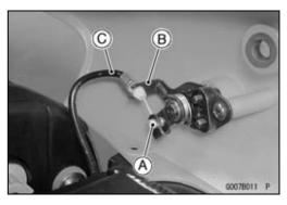
• Remove: Screws [A] Seat Lock [B]
