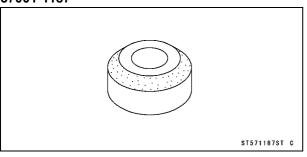
Valve Spring Compressor Adapter,  $\phi$ 22: 57001-1202
