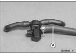
Air Switching Valve Operation Test (ZX1200-B3 ~)
