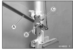
OHolding the piston rod nut [A], remove top plug [B] from the push rod with wrenches.
