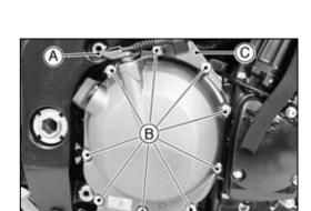
• Turn the release lever [B] toward the rear [C] as shown, and remove the clutch cover [A].
