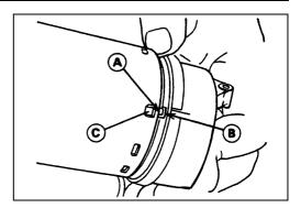
• Align the line [A] marked on the yoke with the through bolt hole [B].
