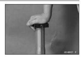
Remove: Spacer [A] Spring Seat [B] Fork Spring [C]
