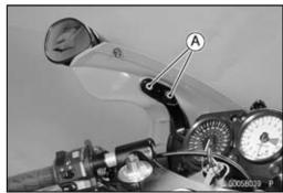
Remove the projections [A] on the left and right upper inner fairings [B] from the grommets [C] on the left and right lower fairings [D] pulling out the lower portion inward of the upper inner fairings.
