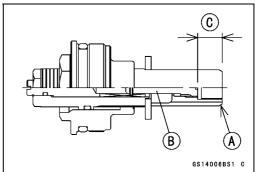
• Set the fork spring compressor on the spacer using the outer tube as a guide.
