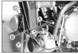
Right Horn Bolt [A] Right Horn [B]
