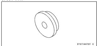
Lead Wire - Voltage Regulator Adapter: 57001-1448
