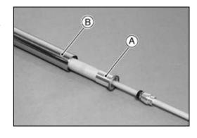
• Install the following parts into the inner tube [A].
