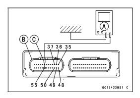
Input Voltage at ECU (Except gear position)
