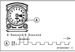
• Insert the user key 1 to the ignition switch and turn it ON.
