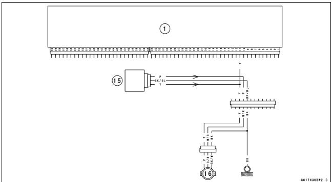
ECU [1] Meter Assembly [15] Speed Sensor [16]
