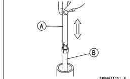
Oil Level (fully compressed, without spring) Standard: 93 ±2 mm (3.66 ±0.08 in.)
