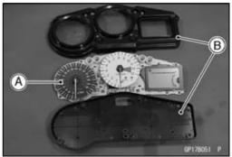
• Remove the screws [A] to separate the inner and outer cover of the upper cover.
