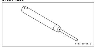
Rotor Puller, M16/M18/M20/M22 × 1.5: 57001-1216
