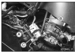
Inlet Air Pressure Sensor Installation
