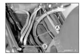
OMove the rear fender front backward until it stops, and then pull downward the right side of the rear fender front [A] to clear the brackets [B].
