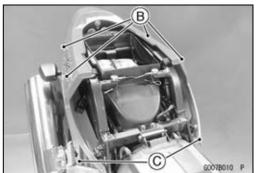
• Pull out the seat lock wire [C] from the bracket [B] to remove the seat lock wire end [A].
