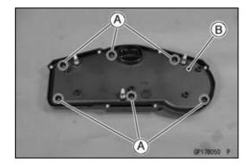
• Separate the meter assembly [A] and meter covers [B].
