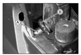
• Remove the alternator leads [A] from the clamps [B].
