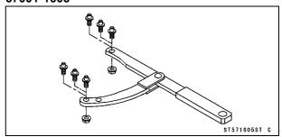
Steering Stem Bearing Driver,  $\phi$ 42.5: 57001-1344
