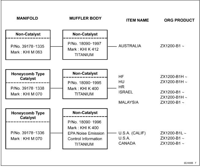
HF: WVTA Approval Model with Honeycomb Catalytic Converter (Full Power Model)
