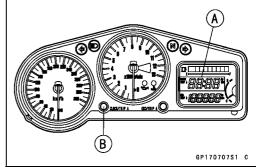
• Check that when the ODO/TRIP B button [A] is pushed within two seconds, the display [B] cycles through the two modes.
