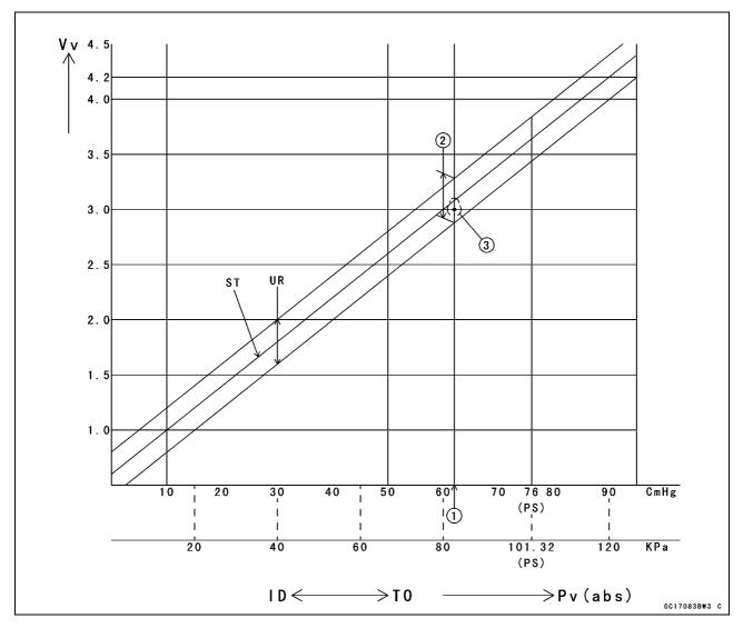
Vv: Inlet Air Pressure Sensor Output Voltage (V)(Digital Meter Reading)
