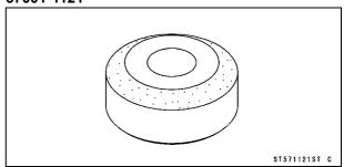
Valve Seat Cutter, 60° -  $\phi$ 30: 57001-1123
