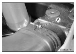
• Remove the nuts [A] and take off the left and right rear view mirrors.
