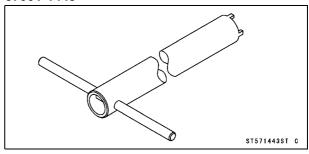
Head Pipe Outer Race Driver,  $\phi$ 55: 57001-1446
