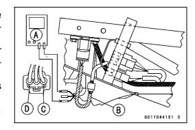
Atmospheric Pressure Sensor Output Voltage Connections to ECU
