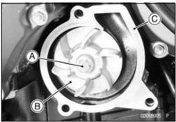
• Remove the water pump housing [B] to hold the water (oil) pump shaft [A] to the crankcase side.
