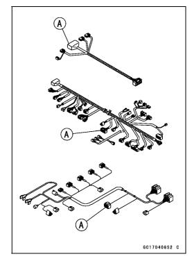
Olf both ends of a harness [A] are far apart, ground [B] the one end [C], using a jumper lead [D] and check the continuity between the end [E] and the ground [F]. This enables to check a long harness for continuity. If the harness is open, repair or replace the harness.
