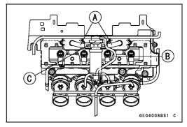
Vacuum Switch Valve Installation (ZX1200-B1/B2)
