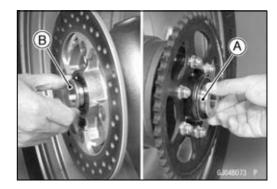
Olf the coupling is removed from the rear wheel, apply the grease as shown.
