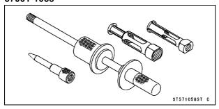
Head Pipe Outer Race Press Shaft: 57001-1075
