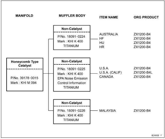
HF: WVTA Approval Model with Honeycomb Catalytic Converter (Full Power Model)
