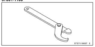
Head Pipe Outer Race Remover ID > 37 mm: 57001-1107
