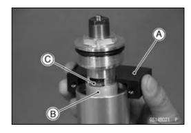
OTighten the bolts [B] to hold the outer tube by using the front fork holder [A], and install the rod [C] to the holder.
