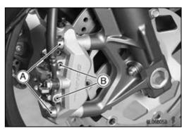
Remove: Pad Pin [A] Pad Spring [B] Brake Pads [C]
