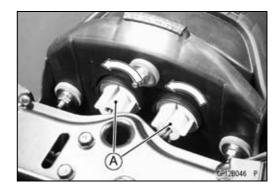
Push and turn the bulb [A] counterclockwise and remove it.
