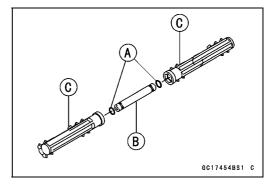
OReplace the O-rings [A] of injectors and the seals [B] with the new ones.
