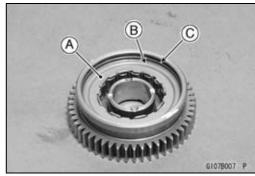
Turn in the driven gear [A] to the drive gear [B].
