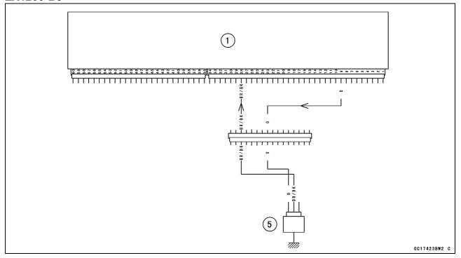
→: Signal ECU [1] Water Temperature Sensor [5]
