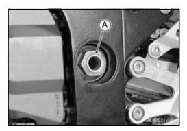
Unscrew the swingarm pivot shaft nut [A].
