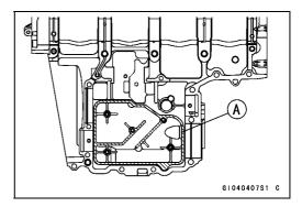
Apply a non-permanent locking agent to the threads and tighten the breather plate mounting bolts [A].
