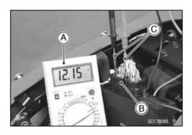
OAfter measurement, remove the needle adapters and apply silicone sealant to the seals [A] of the connector [B] for waterproofing.
