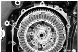
OHolding the clutch hub [A], remove the nut [B] and washer [C]
