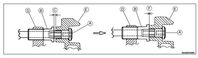
Hold the upper and lower engine mounting bolts with an Allen wrench, and tighten the nuts [A] with specified torque.
