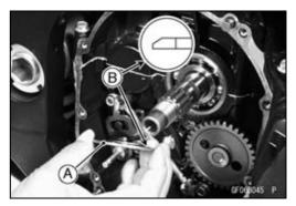
• Install the oil pump drive gear [A] on the clutch housing.
