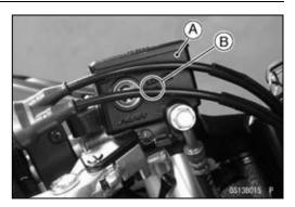
★ If the fluid level is lower than the lower level line, fill the reservoir to the upper level line [A] in the reservoir [B].
