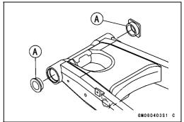
OPlace the right collar [A] on the stopper [B] inside the frame [C].
