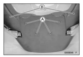
• Take off the screw [A] to remove the air inlet [B].
