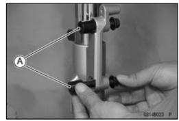
Olnstall the holder plate [A] and lever [B] on these collars with the bolt [C].
