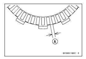
Olnstall the last friction plate [A] fitting the tangs in the grooves in the housing as shown.
