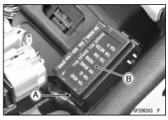
• Pull the sub fuses [A] straight out from the fuse box with a needle nose pliers.
