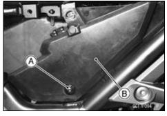
Move the air cleaner housing [A] backward to pull out the air ducts [B] from the throttle body assy [C].
