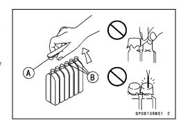
Place the electrolyte container upside down with the six sealed cells into the filler ports of the battery. Hold the container level, push down to break the seals of all six cells. You will see air bubbles rising into each cell as the ports fill.
