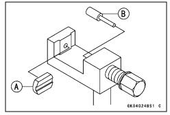
• Turn the pin holder until the riveting pin touches the link pin.
