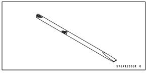
Bearing Remover Head,  $\phi$ 15 ×  $\phi$ 17: 57001-1267
