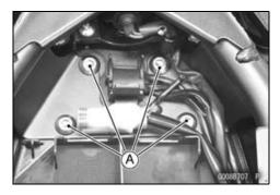
• Install the rubber damper [A] to the frame.
