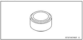
Head Pipe Outer Race Press Shaft: 57001-1075
