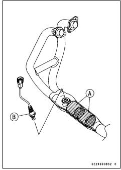
Honeycomb Type Catalyst Positions [A] (without Oxygen Sensor)
