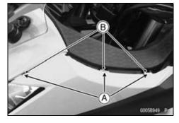
• Insert the tab [A] on the middle fairing into the slot [B] on the upper fairing.
