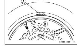
Position the tire on the rim so that the air valve [A] align with the tire balance mark [B] (the chalk mark made during removal, or the yellow paint mark on a new tire).
