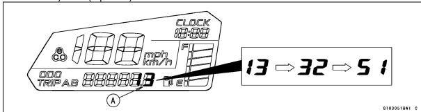
Olf there is no problem or when the repair has been done, the yellow engine warning indicator light (LED) goes off and service code is not displayed.
