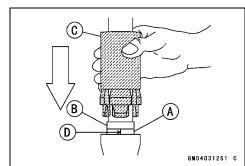
• Apply grease to the oil seal lips, and install the washer and the oil seal [A] into the outer tube.
