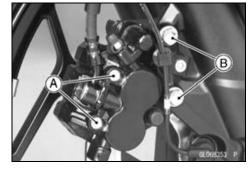
Remove: Pad Pins Brake Pads [A]
