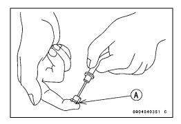
Cables: Lubricate with Rust Inhibitor.
