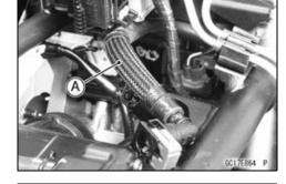
OTo maintain the correct fuel/air mixture (F/A), there must be no intake air leaks in the DFI system. Be sure to install the oil filler plug [A] after filling the engine oil.
