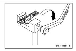
• Set the plate holder (B) [A] and cutting and riveting pin [B] as shown.
