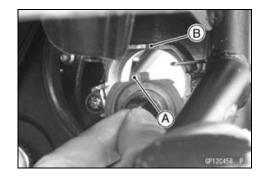
Install the hook [A] and connect the connector [B] to the headlight bulb.
