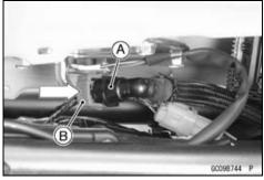
• Push and pull [A] the hose joint [B] more than two times to make sure it is locked and does not come off.
