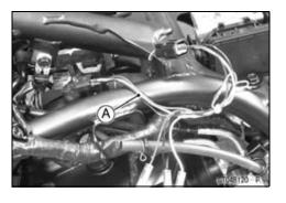
★If the reading is out of the standard, remove the ECU and check the wiring for continuity between main harness connectors.
