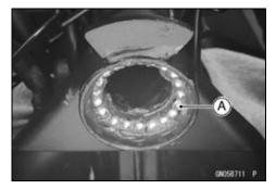
• Apply grease to the upper ball bearings (19) [A] and outer race [B], and install the ball bearings onto the outer race.
