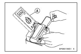
★If the reading is 12.6 V or more, no refresh charge is required, however, if the read is below the specified, refresh charge is required.
