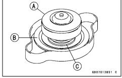
• Install the cap [A] on a cooling system pressure tester [B].
