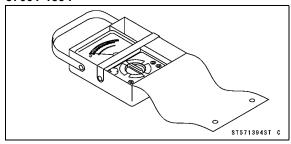
Flywheel Puller Assembly, M38  $\times$  1.5/M35  $\times$  1.5: 57001-1405
