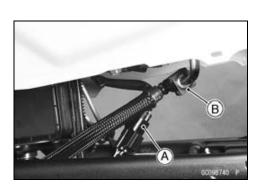
• Wipe off the dirt of the surface [A] around the connection using a cloth or a soft brush.
