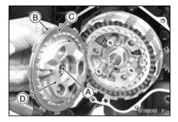
OAlign the tangs [A] on the friction plates (no cutout) with hole [B] on the clutch pressure plate [C] to install them into the clutch housing [D].
