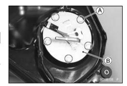
• Remove the fuel pump unit [A] from the fuel tank.
