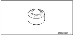
Valve Seat Cutter Holder Bar: 57001-1128
