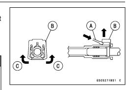
Pull the fuel hose joint [A] out of the outlet pipe [B].
