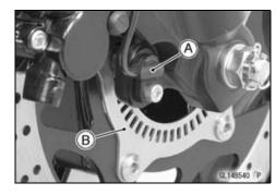
Rear Wheel Rotation Sensor [A] Rear Wheel Rotation Sensor Rotor [B]
