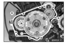
• Install the dowel pins [A] and new gasket [B] are in place on the crankcase.
