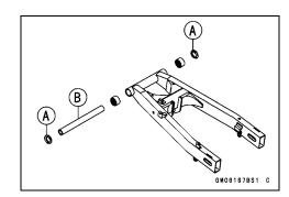
• Remove the needle bearings.
