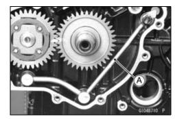
Remove the upper crankcase bolts [A].
