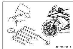
Even when the DFI system is operating normally, the yellow engine warning indicator light (LED) may go on under strong electrical interference. Additional measures are not required. Turn the ignition switch off to stop the indicator light.
