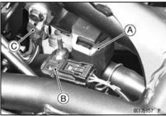
Water Temperature Sensor [A] Vehicle-down Sensor [B]
