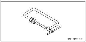
Piston Pin Puller Assembly: 57001-910
