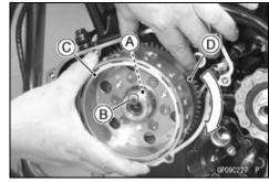
• Install the washer [A] with its chamfer side [B] facing out.
