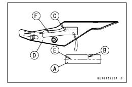
• Insert the claw [A] into the cover clamp [B] and tighten the clamp screw [C] as shown.
