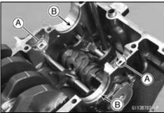
• Install the drive shaft and output shaft into the upper crankcase half aligning the followings:
