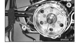
• Using the flywheel puller [A], remove the alternator rotor [B] from the crankshaft.
