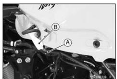
For models equipped with the evapratice emission control system, disconnect the fuel tank drain hose [A] and breather hose [B] from the fuel tank.
