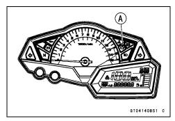
With the engine stopped and turned in the self-diagnosis mode, the service code [A] is displayed on the LCD (Liquid Crystal Display) by the number of two digits.
