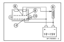
• Check that the number of segments [A] matches the resistance value of the variable rheostat.
