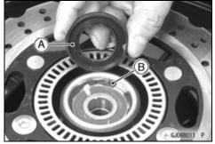
• Use the bearing remover to remove the hub bearings [A].
