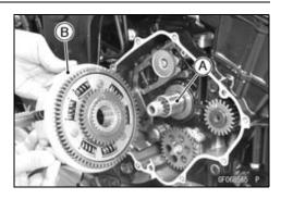
OHolding the clutch hub [A], tighten the clutch hub nut [B]. Special Tool - Clutch Holder [C]: 57001-1243
