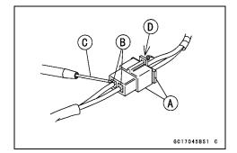
OAfter measurement, remove the needle adapters and apply silicone sealant to the seals [A] of the connector [B] for waterproofing.
