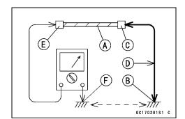
OWhen checking a harness [A] for short circuit, open one end [B] and check the continuity between the other end [C] and ground [D]. If there is continuity, the harness has a short circuit to ground, and it must be repaired or replaced.
