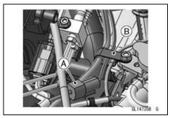
Clear the sensor lead from the clamp [A].
