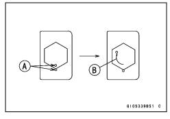
OThe nuts can be tightened by using a torque angle gauge [A].
