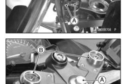
Pushing up the stem base, and remove the steering stem nut [A] and stem cap [B].
