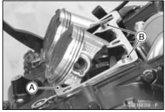
The piston ring openings must be positioned as shown.
