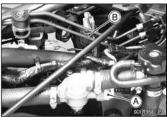
Intake Air Temperature Sensor [A]
